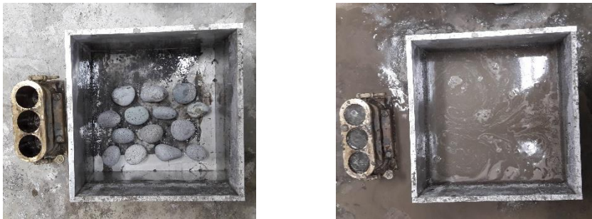
Fig. 2. Preparation of grouted gravel specimens in this study
